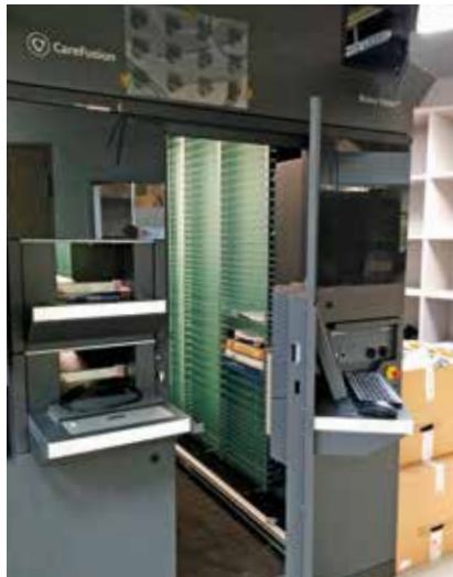
Figure 69 A ROWA machine picks boxes of medications.
